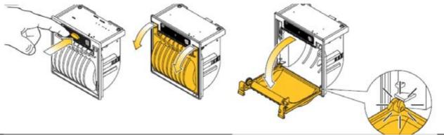
2. Place the paper roll making sure that it unrolls in the proper direction as shown.
