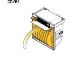
4. Push on the plastic cover to lock it and tear off the exceeding paper using the jagged edge.
